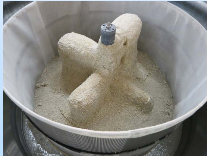
sandpack around simulated perforations high P
