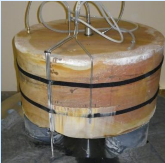
30 cm radial fracture high P
